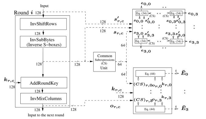
Fig. 7. The proposed low-complexity fault detection scheme for the  $i$ th round of the AES decryption utilizing subexpression sharing.
