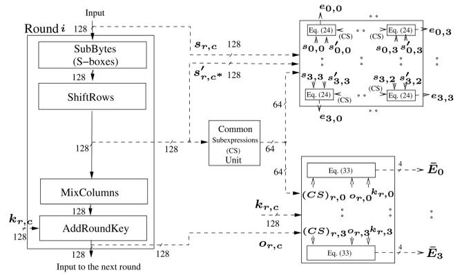
Fig. 5. The proposed low-complexity fault detection scheme for the  $i$ th round of the AES encryption utilizing subexpression sharing.
