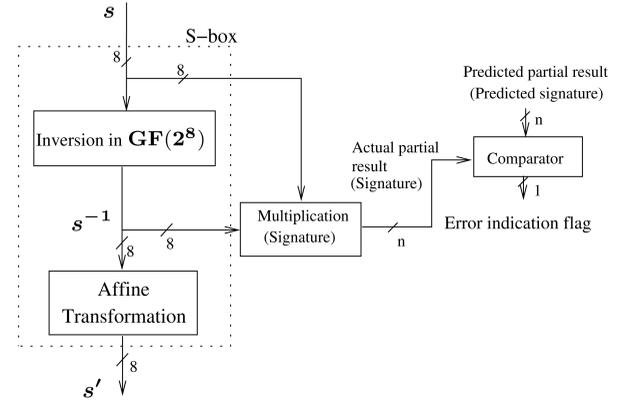
Fig. 1. The multiplication-based scheme for the fault detection of the multiplicative inversion [19].
