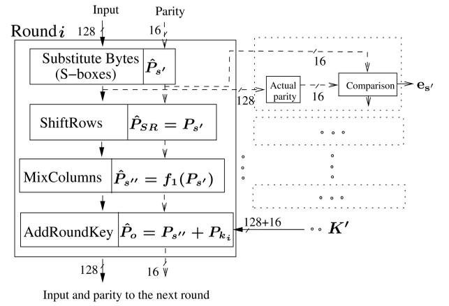
Fig. 3. Recursive parity-based fault detection structure of the  $i$ th round for encryption in AES [8].
