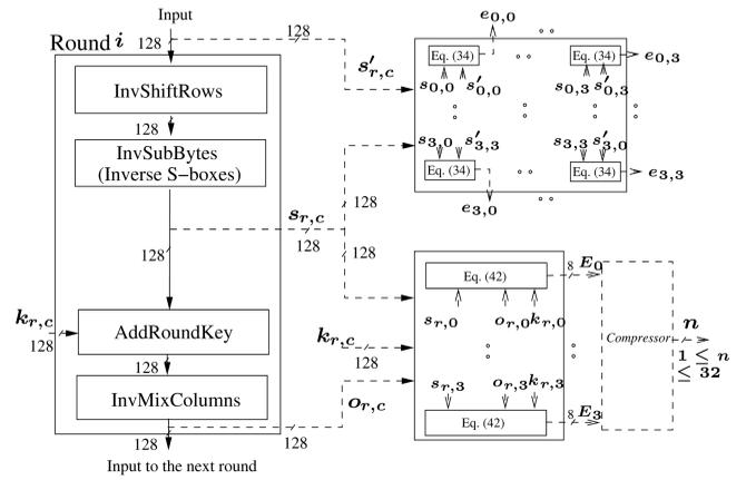
Fig. 6. The proposed fault detection scheme for the  $i$ th round of the AES decryption.
