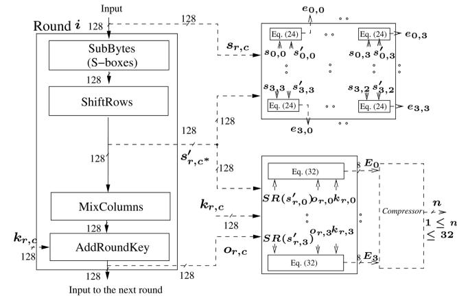
Fig. 4. The proposed fault detection scheme for the  $i$ th round of the AES encryption.
