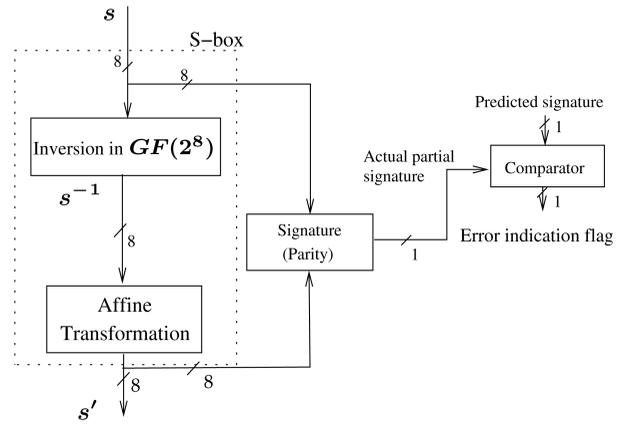
Fig. 2. The proposed structure-independent fault detection scheme of the S-box.
