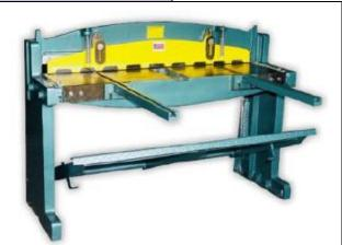
**Potential Hazards:** Exposed blade with significant mechanical advantage when handle is pulled. Exposed moving parts and gears. Extreme cutting hazard is always present. Risk of cuts from sharp work piece edges after every cut.
